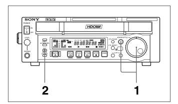
**1** Holding down the JOG/SHUTTLE button, turn the JOG/SHUTTLE dial.
